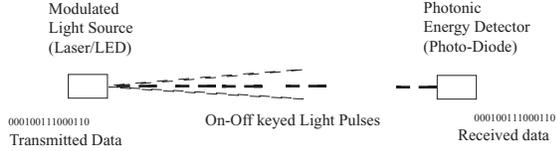
Fig. 1. Typical single hop FSO communication system.
