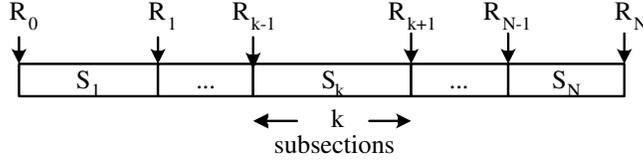
**Figure 9.** Rate partition of an embedded bitstream into  $N$  layers or quality levels
