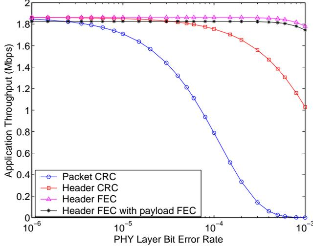
Figure 4. Application layer bandwidth efficiency vs BER
