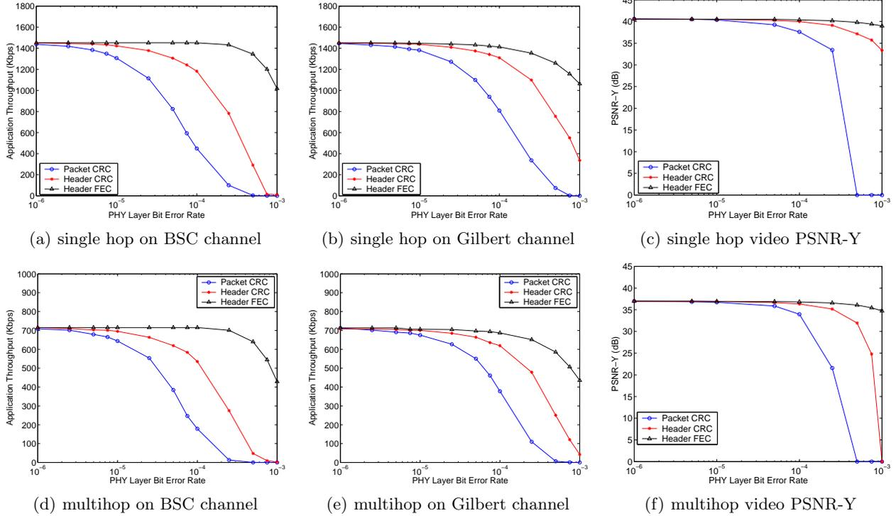
**Figure 12.** Effective application layer throughput on BSC and Gilbert channel at different physical layer BER and corresponding Video PSNR\_Y
