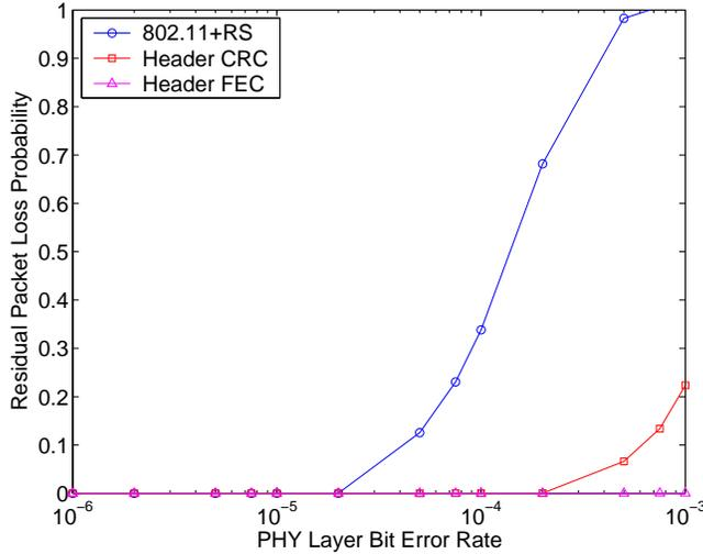
**Figure 6.** Residual packet loss probability of several FEC schemes vs BER
