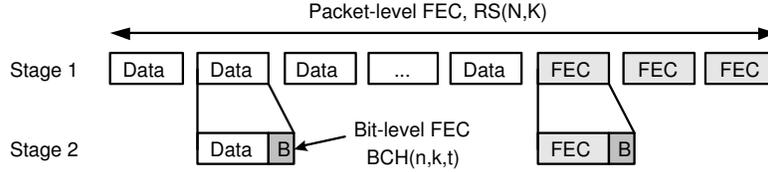
Figure 5. Detail of the proposed two-stage FEC scheme
