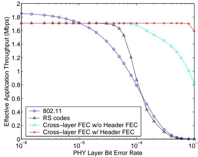
**Figure 7.** Effective application layer throughput efficiency of several FEC schemes vs physical channel BER
