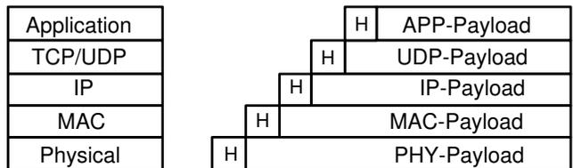
Figure 1. 802.11 protocol stack and associated packet structure
