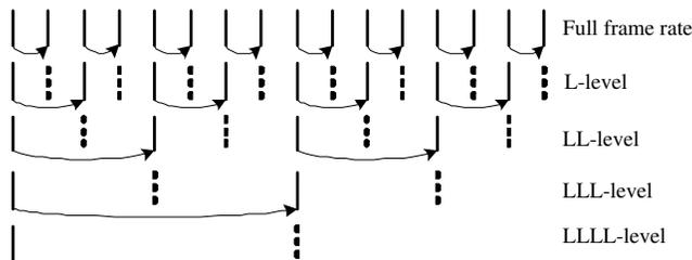
**Figure 8.** A typical GOP of 16 frames with 5 layers of temporal scalability
