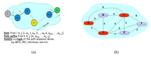
Figure 1: Figure showing (a) Path, PathSuffix and PathID Concepts (b) Multi-Path Forwarding with Partial Upgrades
