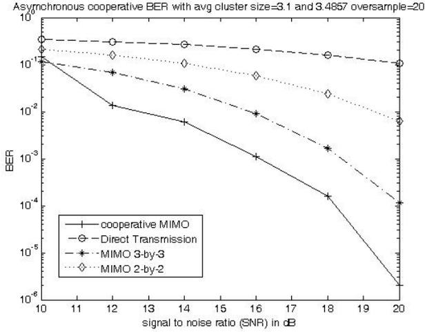
Fig. 4. BER performance comparison of proposed system with typical MIMO systems and direct transmission (Note: over-sampling rate=20, average cluster size is 3.1 for transmitting cluster and 3.49 for receiving cluster respectively.)
