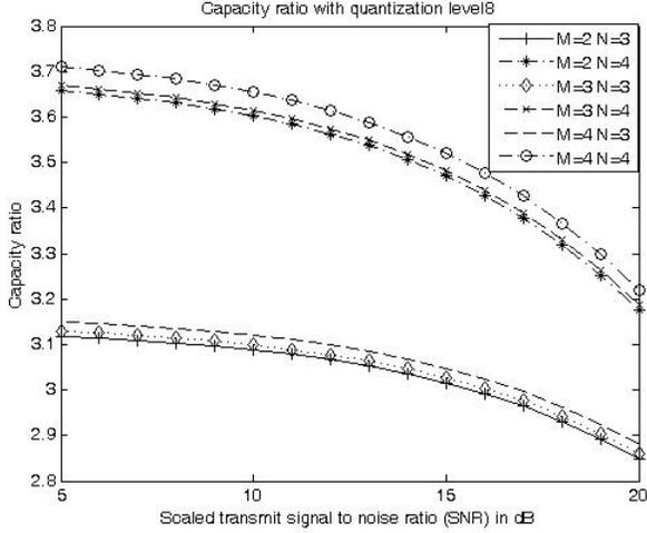
Fig. 6. Capacity ratio of different transmitting/receiving cluster size with scaled SNR. (Note: scaled SNR is defined as  $P_T/r^\alpha$ ,  $r$  is cluster radius and  $P_T$  is transmission power)
