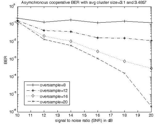
Fig. 5. BER performance with different oversampling rate
