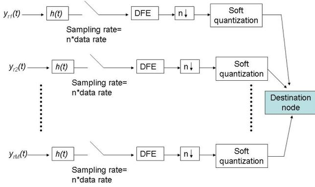
Fig. 3. Signals in each destination cluster member are processed by match filter and DFE before soft symbol quantization. The quantized soft symbols are sent to destination node.
