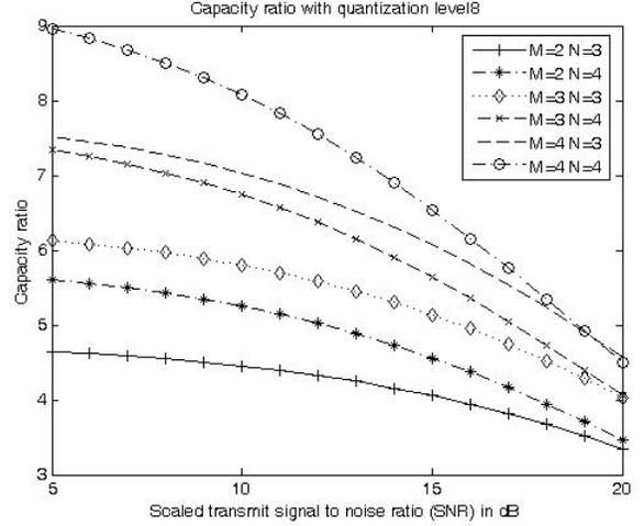
Fig. 9. Capacity ratio with scaled SNR (Note: each node has 2 antenna)
