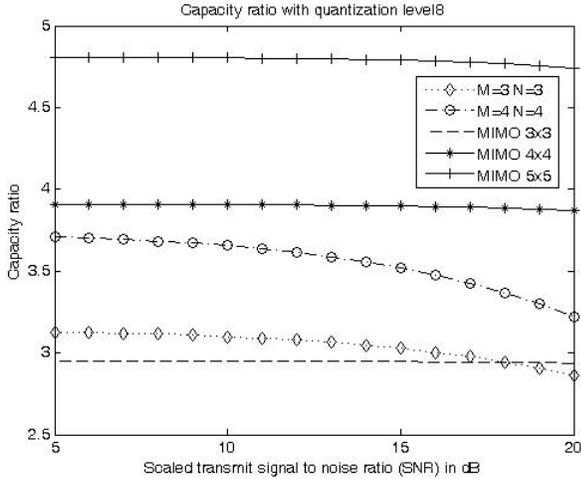
Fig. 7. Capacity ratio compared to conventional MIMO system with scaled SNR (Note: scaled SNR is defined as  $P_T/r^\alpha$ ,  $r$  is cluster radius and  $P_T$  is transmission power)
