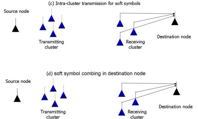
Fig. 2. Proposed cooperative scheme: (c) Relaying copies to destination node. (d) soft symbol combining
