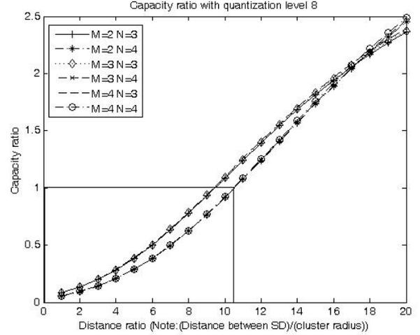
Fig. 8. Capacity ratio with distance ratio (Note: scaled SNR is defined as  $P_T/r^\alpha$ , where  $r$  is cluster radius and  $P_T$  is transmission power. Distance ratio is defined as  $d_{SD}/r$ , where  $d_{SD}$  is distance between source and destination node)
