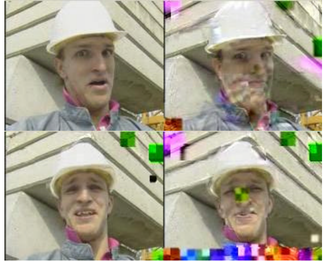
Figure 6: Sample frames from the video streaming experiments: OM-FEC (left) vs. End-to-End FEC (right) over 4 virtual links (top) and 5 virtual links (bottom).
