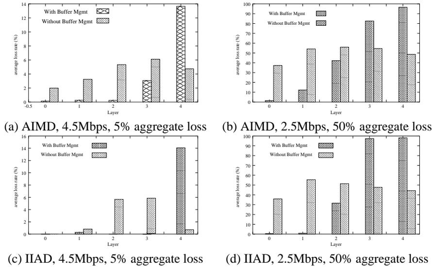
Fig. 5. Comparison of average loss rates per layer with and without buffer management
