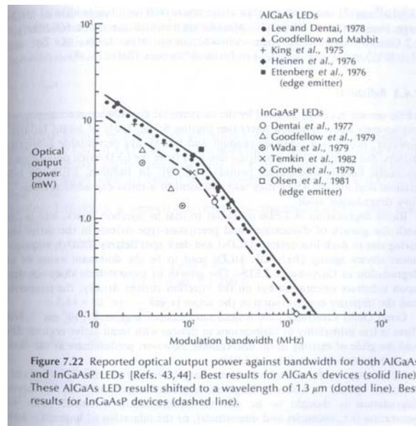
Figure 7.22 Reported optical output power against bandwidth for both AlGaAs and InGaAsP LEDs [Refs. 43, 44]. Best results for AlGaAs devices (solid line). These AlGaAs LED results shifted to a wavelength of 1.3 μm (dotted line). Best results for InGaAsP devices (dashed line).
