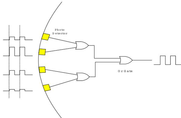
**Figure 7: Open-Loop OR-gate Design For LOS-Discovery (Op-Amps, Filters omitted for simplicity).**
