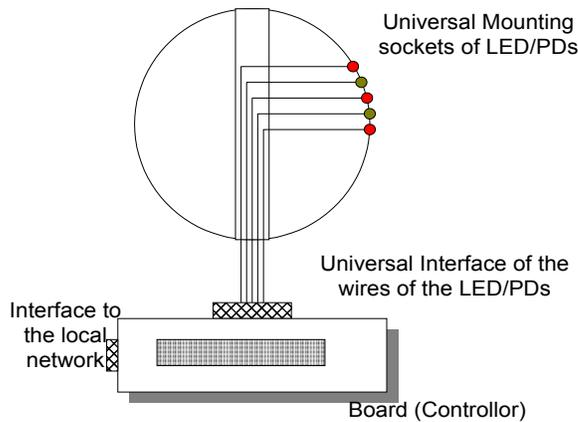
**Figure 5: Current Design of Optical Antenna**
