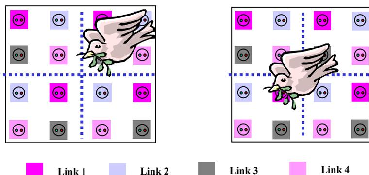
**Figure 8: Spatial Error Coding to Protect against Temporary Obstacles**
