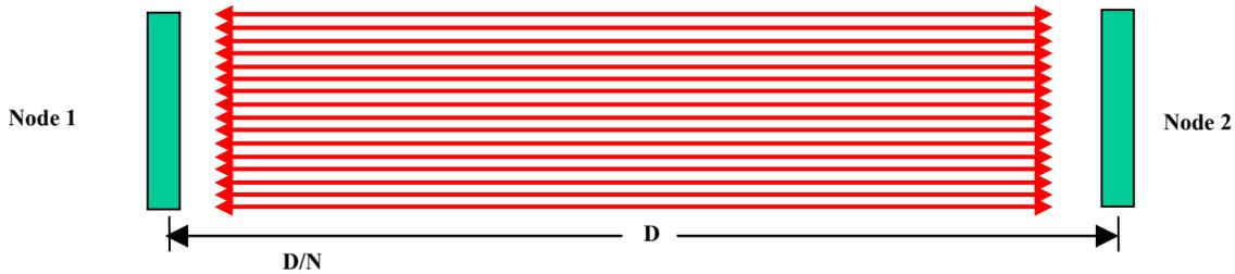
Figure 3: Two-dimensional FSO Transceiver Array for Dense Spatial Bandwidth Re-use
