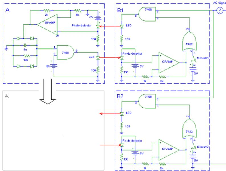
**Figure 6: Simplified “Feedback” Design for Automatic LOS Discovery and Alignment**
