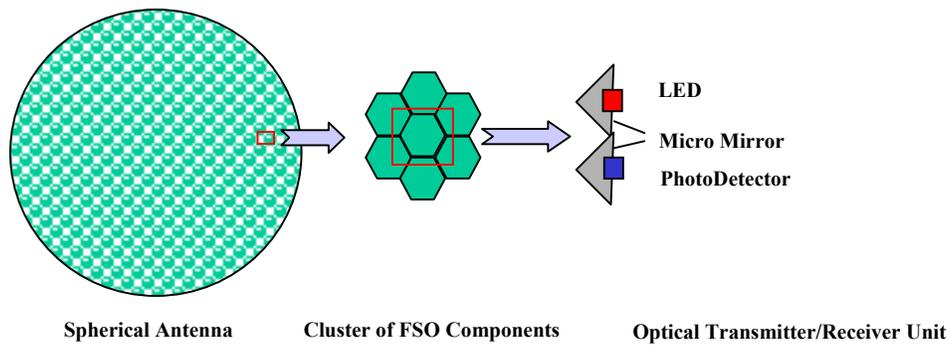
Figure 1: Optical Antenna: 3-d Honeycomb Structure
