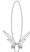
**Figure 1: Radiation Pattern for Directional Antennas**
