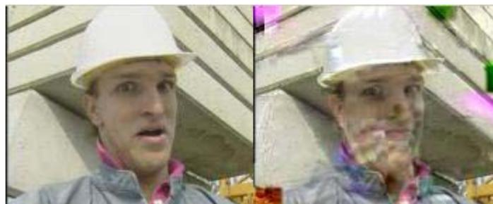
Figure 11: Video streaming over 4 virtual links: OM-FEC (left) vs. end-to-end scheme (right).
